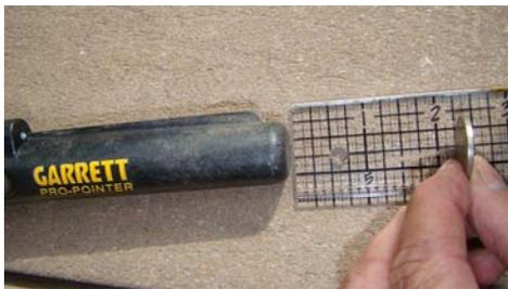
I tested (tried to test) the depth ability of the 3 pinpointers on 4 separate occasions. The results were discouragingly inconsistent, both during each test, and as compared to other tests. Never-the-less, it appears the White's TRX obtained more depth than either of the Garrett's, but this advantage can be mitigated to a widely varying degree by using the Garrett Coin Slide. This is a neat little trick most of the
